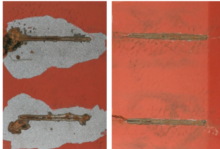
Scribe Test comparison: Commercially available liquid-epoxy based coating vs AMP-UP™ 100 (2000 hrs in salt spray chamber ASTM B117)
